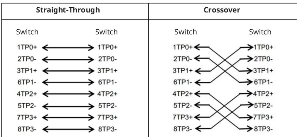
100BASE-TX/10BASE-T can be interconnected using cables of the preceding specifications. For 10 Mbps, the 100BASE-TX/10BASE-T port can be connected using 100-ohm Category 3, Category 4, and Category 5 cables; for 100 Mbps, the 100BASE-TX/10BASE-T port can be connected using 100-ohm Category 5 cables with a maximum connection distance of 100 meters. The following table shows 100BASE-TX/10BASE-T pin assignments.
