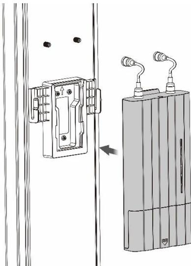
(3) Connect the SMA connector of the wireless bridge to that of the antenna.
