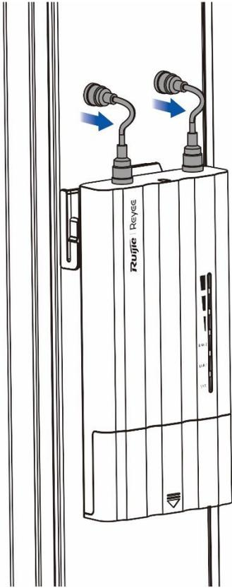
(3) Remove the wireless bridge by pulling it upward and then outward.
